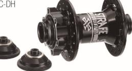
R-142 + QR XC-FR 142mm rear hub is alternative with 135mm QR side caps which are included in the package, as well as the free hub body is alternative of optional parts SRAM XX1 cassette body (with XX1 specialized caps).
