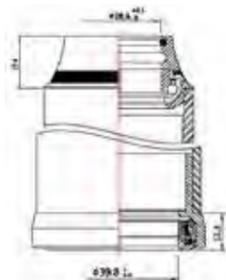
**1.5" TAPERED INTEGRATED OUTER BEARING DESIGN (ZS44/EC49)**
